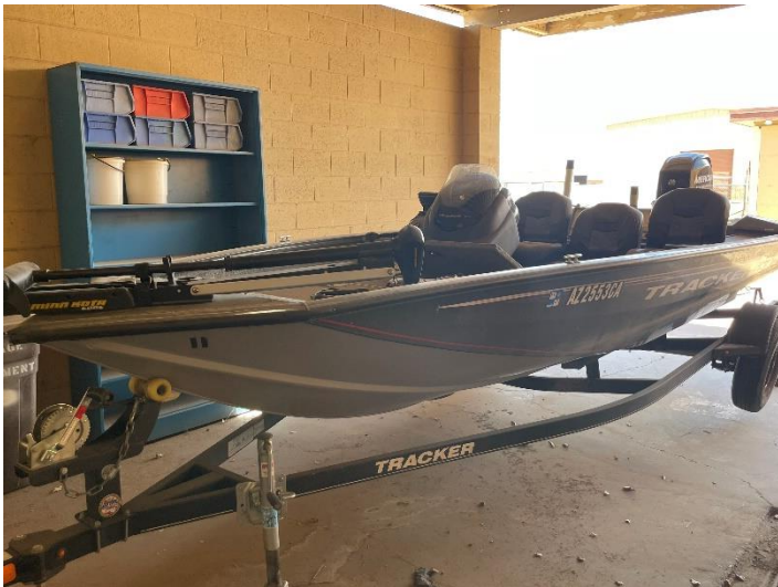
Boat #11- 17' Tracker Bass Boat, 4 Person (4seats, 3seats while moving), 60HP, Trolling Motor, Wheel Steering
